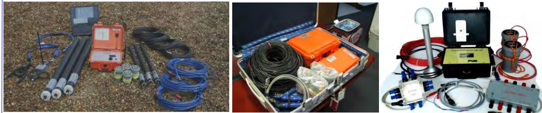
KMS-200 software works with KMS-820 MT system (left), Mini Mt system (middle), LEMI-424 system (right)
