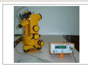
Inclinometer/declinometer installed in non-magnetic theodolite
