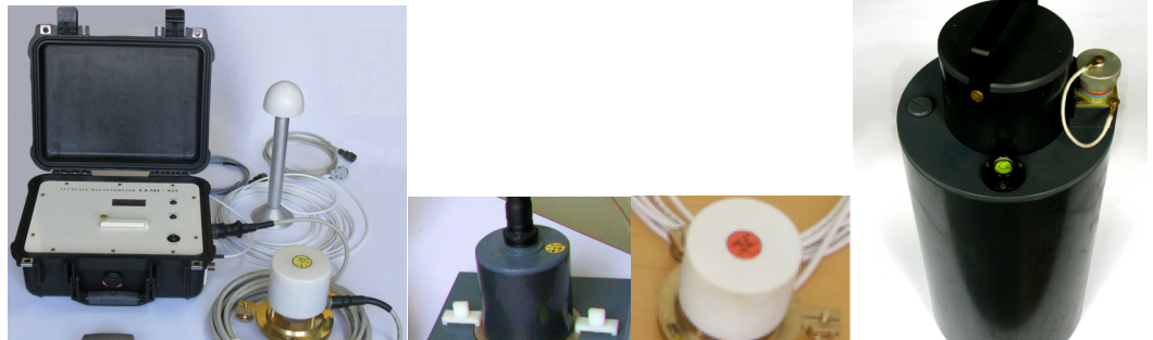
Figure 1: LEMI-025 system with sensor in various options. The suspended option is shown on the right
